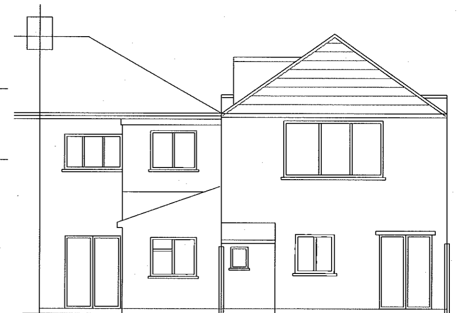
EXISTING REAR ELEVATION
